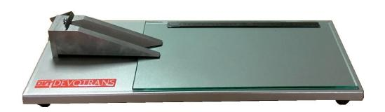
PERMET DE TESTER DES ADHESIFS EN MESURANT LA DISTANCE PARCOURUE PAR UNE BOULE ROULANTE AVANT DE S'ARRETER
